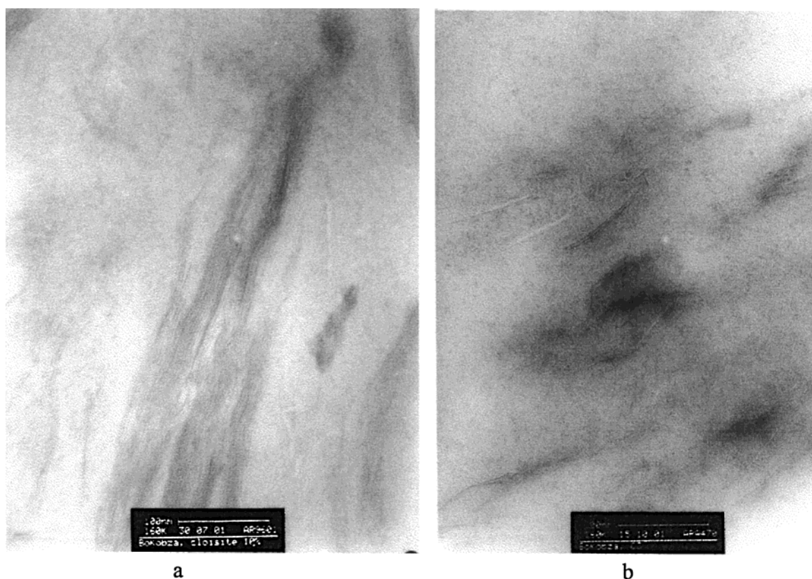
Figure 3. TEM micrographs of natural rubber filled with 10 wt % of clay: (a) is for pristine clay (Na-Mt) and (b) is for organo-modified clay (M3). The higher horizontal bar corresponds to 100 nm.
